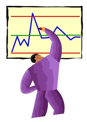
A time-ordered plot of process data points with a centerline based on the average and control limits that bound the expected range of variation
