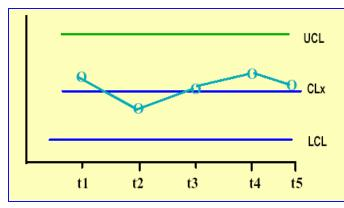
Process is not stable ("Out-of-control" Process)
